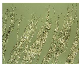
A wear debris sample, generated by the ANALEX<sub>rpd</sub> and viewed under a microscope.
