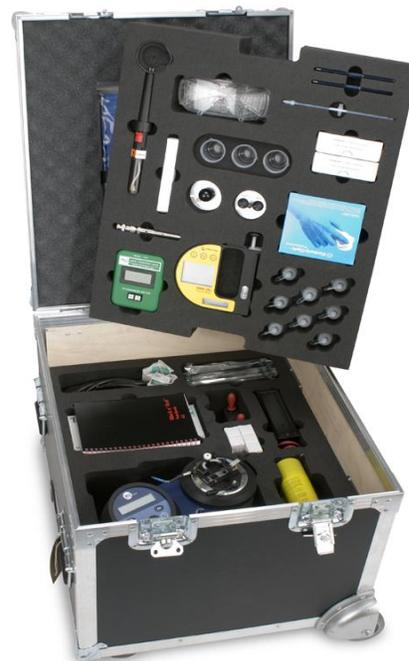
**Flash Point.** A Setaflash Series 3 Closed Cup Flash Point Tester provides either a go/no-go test, or can determine the actual flash point of the sample. The Setaflash is a laboratory standard instrument featuring an automatic flash detection system that provides a result in two minutes. A power inverter is included to allow operation from a 12V dc supply.
